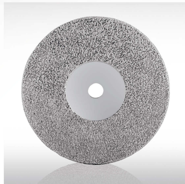
FLB034 Grit: #30, #50 Diameter: 4", 5" Connection: M14 or 5/8"-11
