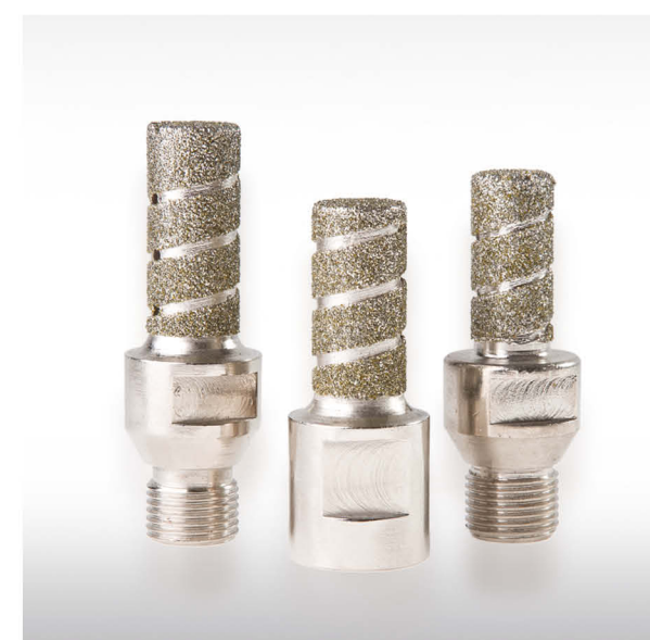
FLE234 Grit: #30 Diameter: 16/18/20/25mm Connection: M14 or 1/2" GAS
