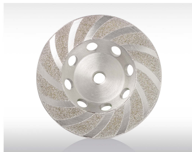
FLE088 Grit: #40 Diameter: 100mm, 115mm, 125mm Hole: 22.23mm Connection: M14 or 5/8"-11
