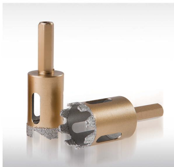
FLB008T Professional used on around 3cm thick granite with low RPM Diameter: 16~120mm Shank: hexagon or 1/2" GAS Wet/Dry drilling: Wet RPM: 1000RPM Drill machine: bench drill machine
