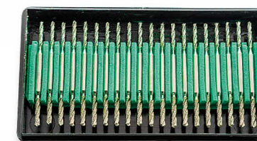
FLE040 Grit: #120/140 Shank dia.: 3.175mm Head dia.: 1.6mm and 2.1mm Total length: 46mm Application: jade, glass and other hard brittle materials hole processing
