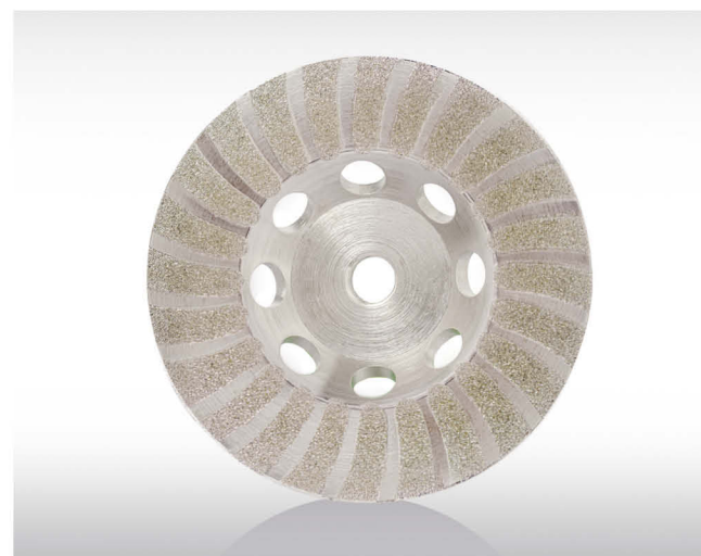
FLE086 Grit: #40 Diameter: 100mm, 115mm, 125mm Hole: 22.23mm Connection: M14 or 5/8"-11
