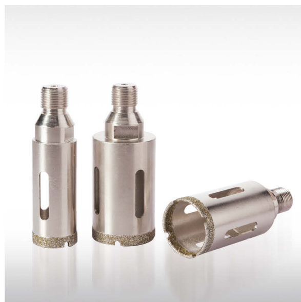
FLE09908 Grit: #30 Diameter: 16~150mm Shank: 1/2" GAS thread
